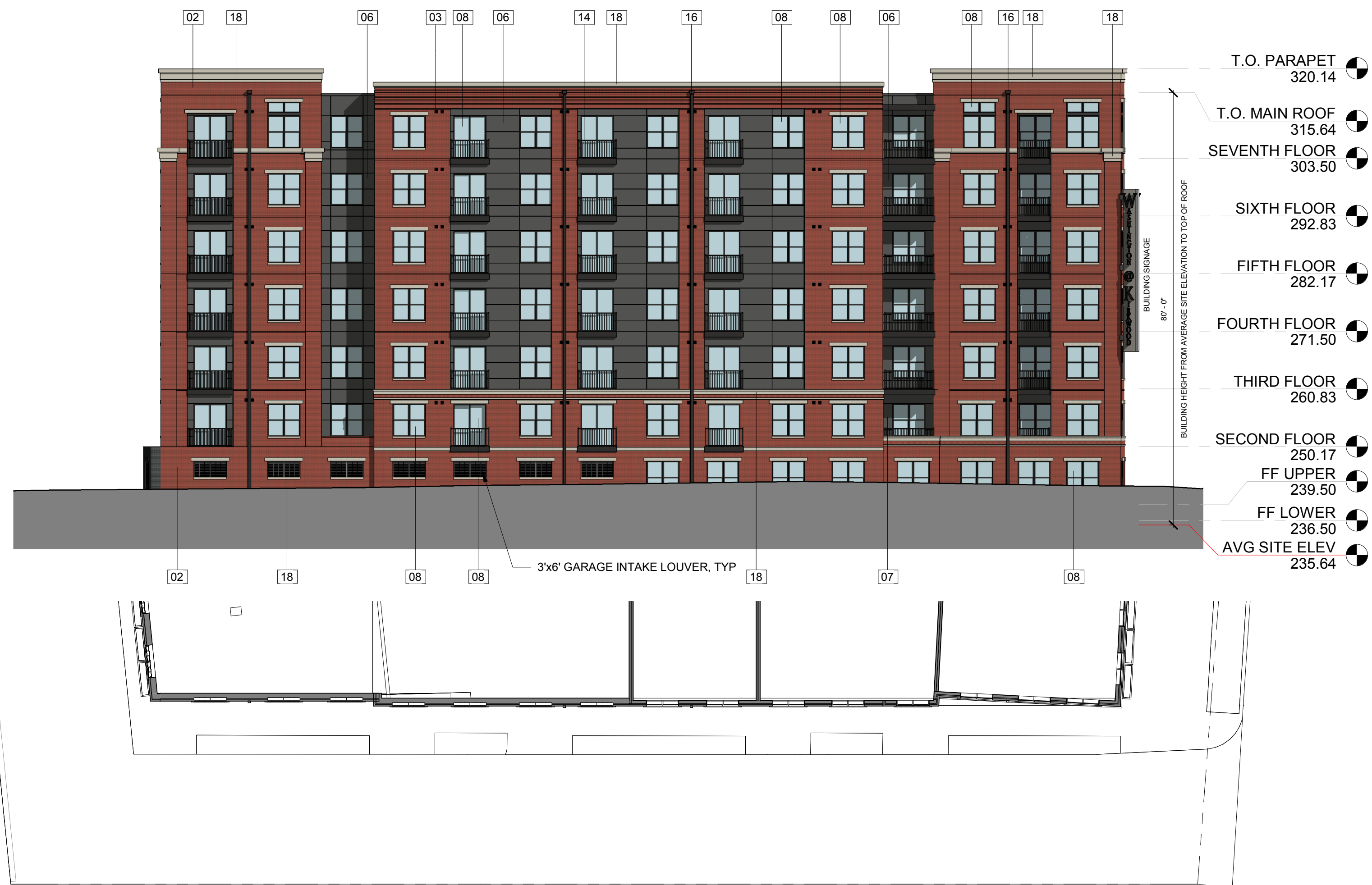
2 BUILDING ELEVATION - WEST ALLEY 1/16" = 1'-0"
