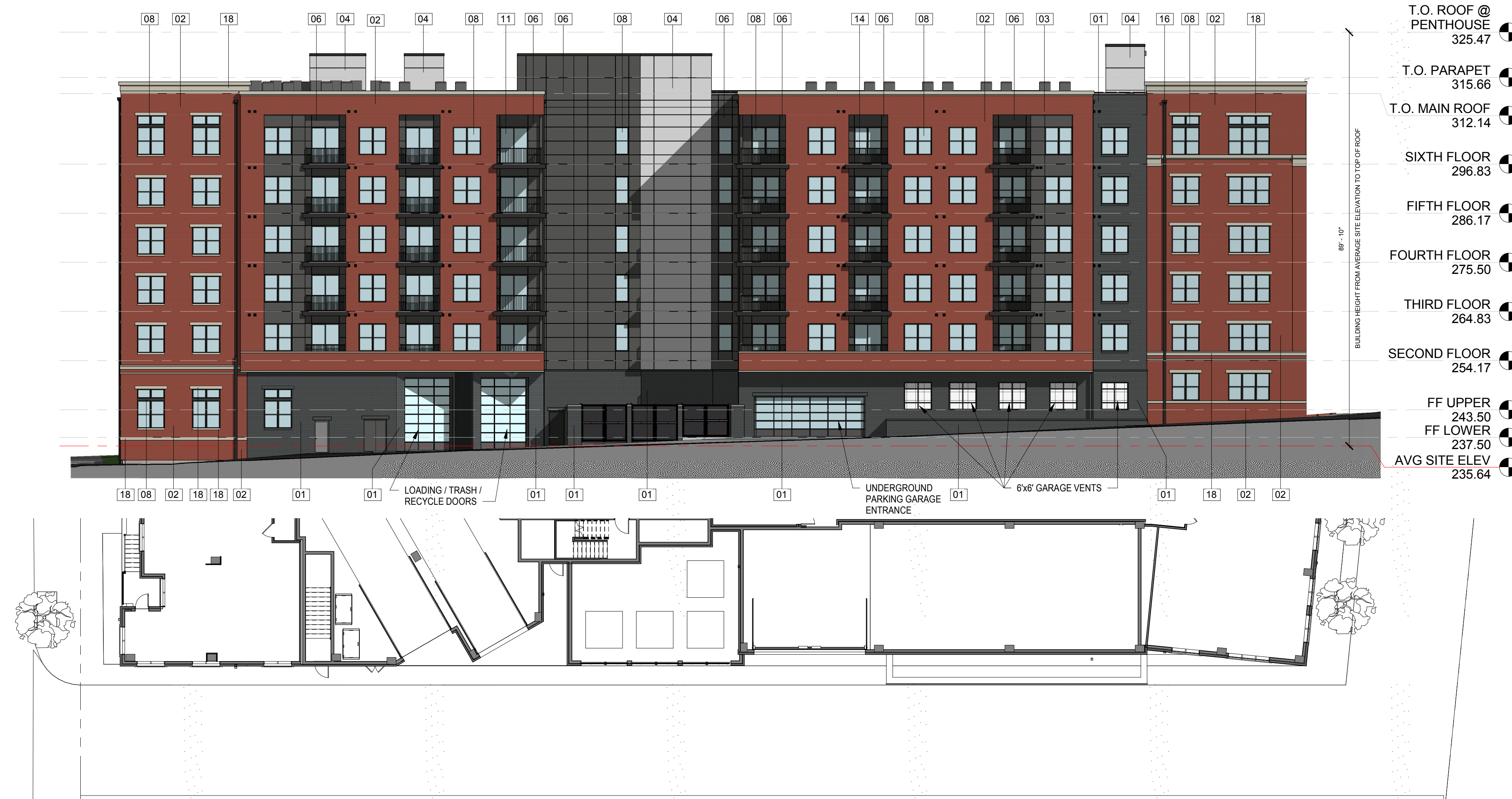
1 BUILDING ELEVATION - NORTH ALLEY 1/16" = 1'-0"
